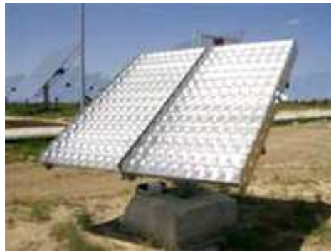
Figura 12: Fresnel point focus.
