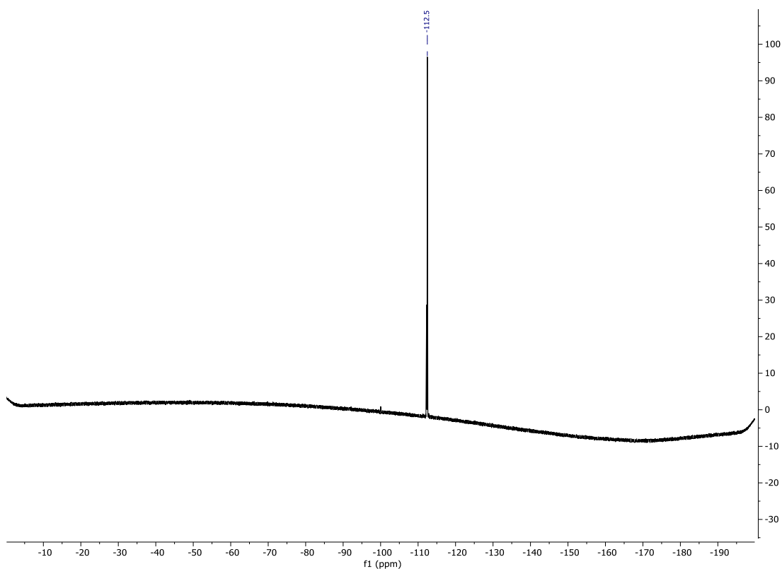
Figure 2.36. ^{19}\text{F}\{^1\text{H}\} NMR spectrum of compound 62 in DMSO solution.
