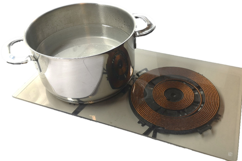
Fig. 5.40 Inductor-load system composed of two series 21-cm inductors and two zenith pots. Its equivalent series resistance is 10.5 \Omega whereas its equivalent series inductance is 57 \mu H.
