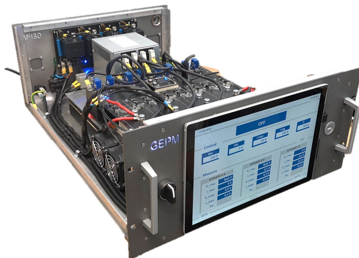
Fig. 5.10 Complete system of the three-phase bidirectional power supply in a custom-made 5U rack along with the user interface.
