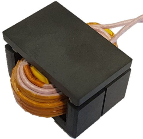
Fig. 5.28 Implemented boost and balancing inductors for HS modulation strategies. It features 110- \mu\text{H} inductance and 55-A saturation current. The dimensions are 4.3 cm, 4.7 cm, and 2.8 cm, obtaining a 57- \text{cm}^3 volume. The maximum power losses operating at 11 kW are estimated in 13 W.
