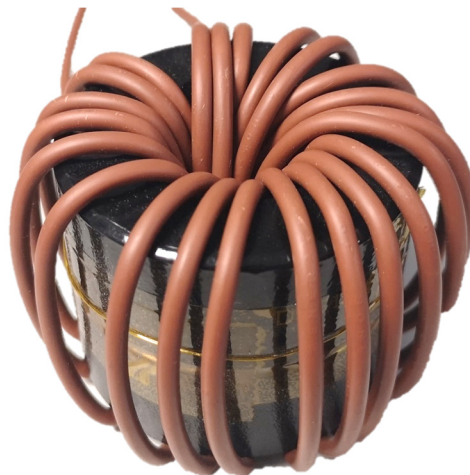
Fig. 5.15 Boost inductor for HS CCM modulation strategies.
