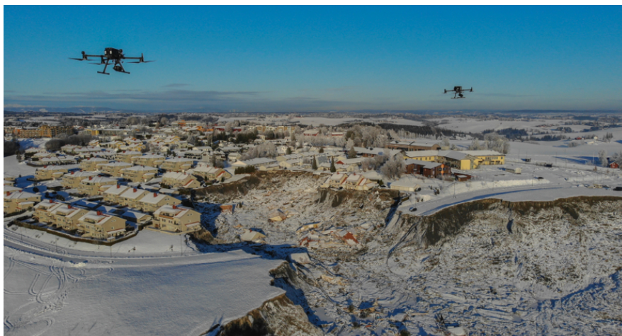
Figure 1.1: Use case of a team of drones for disaster surveying during Gjerdrum landslide in Norway 1 . Drones can traverse large distances fast and reach inaccessible areas.
