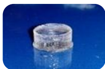
Figure 10. Obtained photopolymerized hydrogel after demould it. Material: P/A-2, 23% (w/v).
