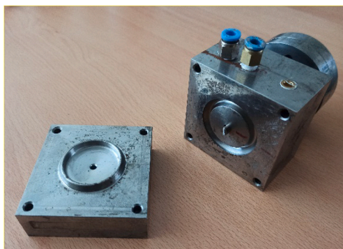
Fig. 1. a: Samples of recycled HDPE studied. b: Sketch of the body (left), and of the lid (right) (Dimensions in mm). c: Lid (left) and body (right) molds.
