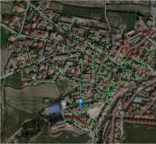
Fig. 6. Image of the optimal location of the EV charger compensating voltage unbalances in the Southern Europe rural grid.
