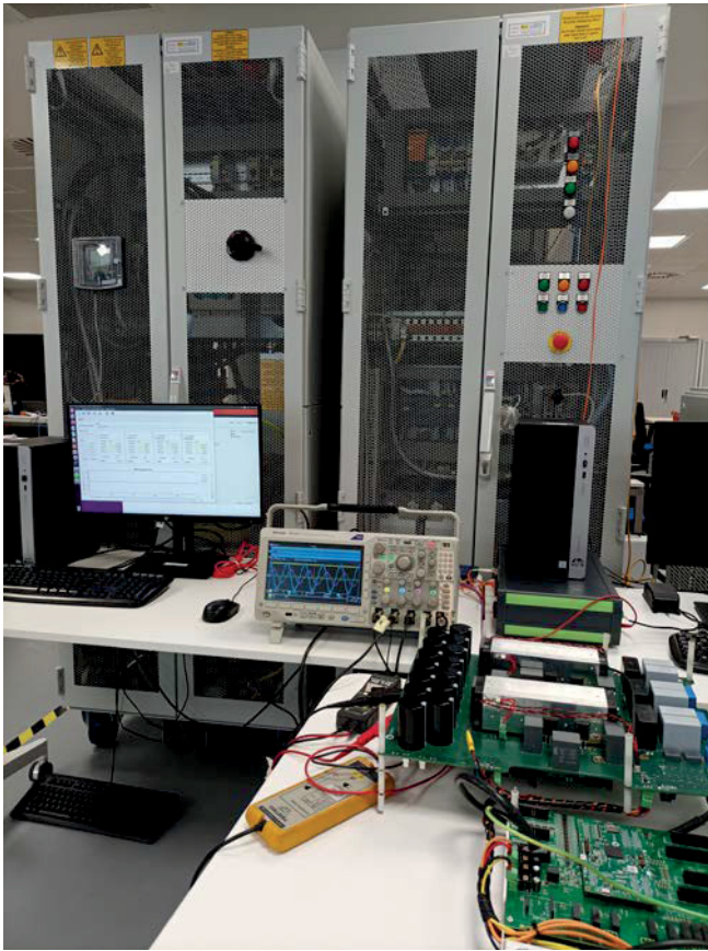
Fig. 2.: AC/DC converter tested with PHIL in CIRCE Laboratory.
