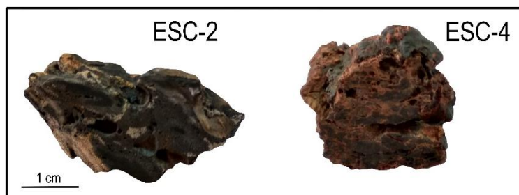
Fig 7.1. Images of a black natural clinker sample with yellow areas (ESC-2) and another red with black areas (ESC-4).
