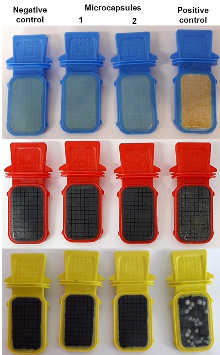
Figure 80. Photographs of sterility testers analysing the presence of microorganisms, comparing a negative control (sterile water), two different batches of microcapsules with AuNPs (microcapsules 1 and 2) and a positive control of contamination (ground sample). Coliform organisms were tested using the Coli-Count™ Sampler (blue), aerobic bacteria
