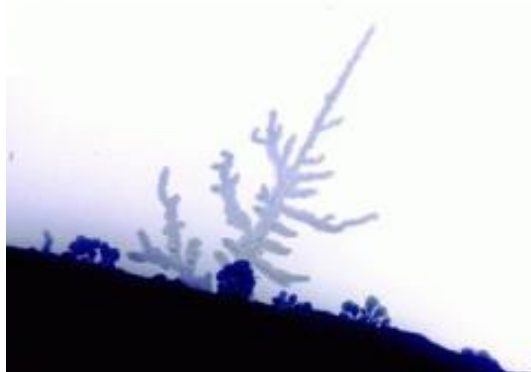
Figure 4. Optical microscope image of a Li dendrite [30].
