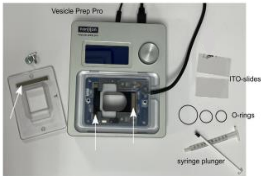
Fig. 10: Vesicle Prep Pro device and its components. White arrows mark the electrodes, which are touching conductive sides of the ITO-slide (14) .
