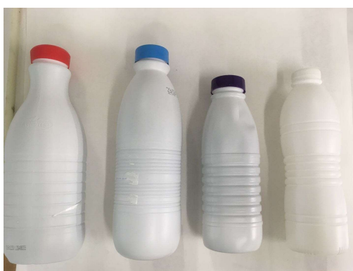
Fig. III-4.2 Self-collected HDPE bottles (the last one is the package of liquid yogurt while the others are the packages of milk)
