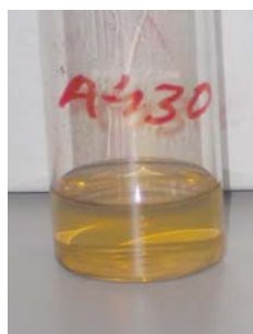
Figure 3.11 Photograph of iron oxide nanoparticles coated with TEOS stabilized in water.
