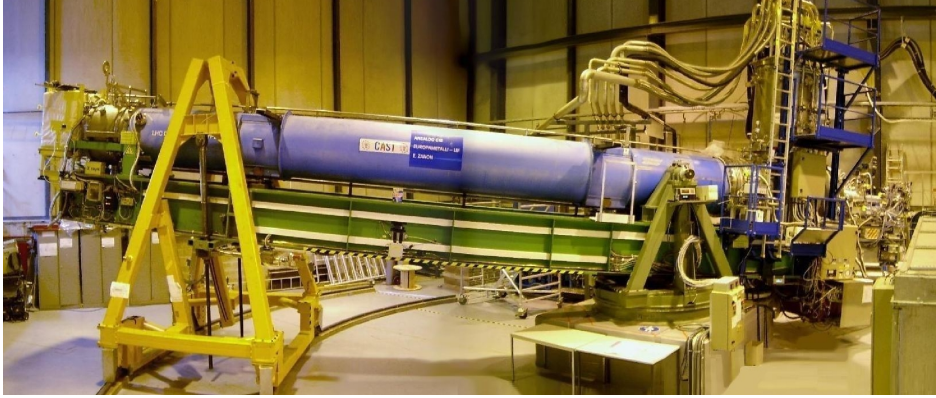
Figure 8.1: Picture of the CAST helioscope, a materialization of the principle represented in figure 1.9. Detectors are installed at both magnet ends, two face the sun during sunrise (in the photo on the right) and the other two at sunset (on the left).
