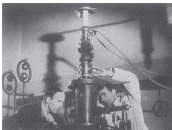
Figure 1.1: The electron microscope built by Ruska and Knoll in Berlin in the early 1930s. Source: [2].
