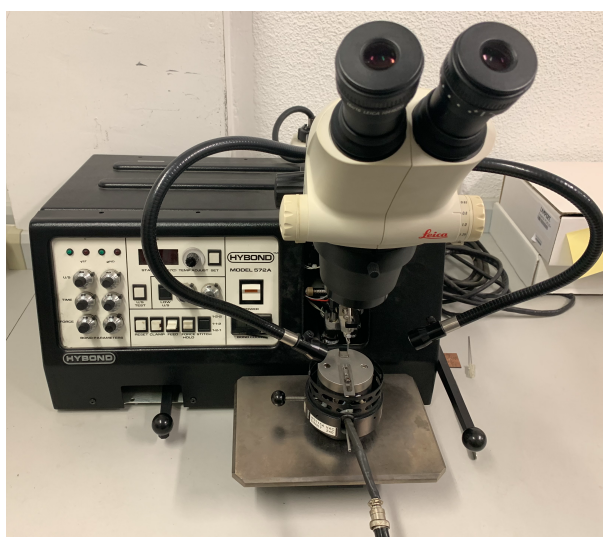
Figure 2.23: Hybond model 572A wire bonding machine at the INMA.
