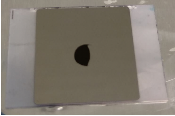
Figure 4.33: Photo of the third DPPH deposition, performed with micropipette on the 2.5D resonator with a 50 nm wide nanoconstriction. The ink used here had a DPPH concentration of 80 mg/ml.
