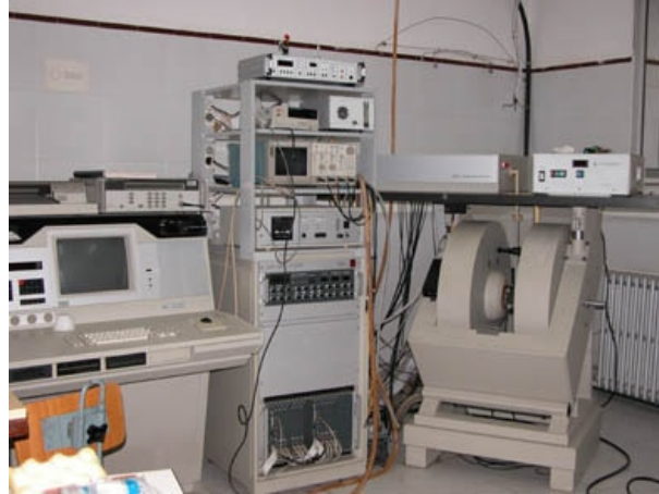
Figure 2.12: Eleksys E-580 EPR spectrometer at the University of Zaragoza.
