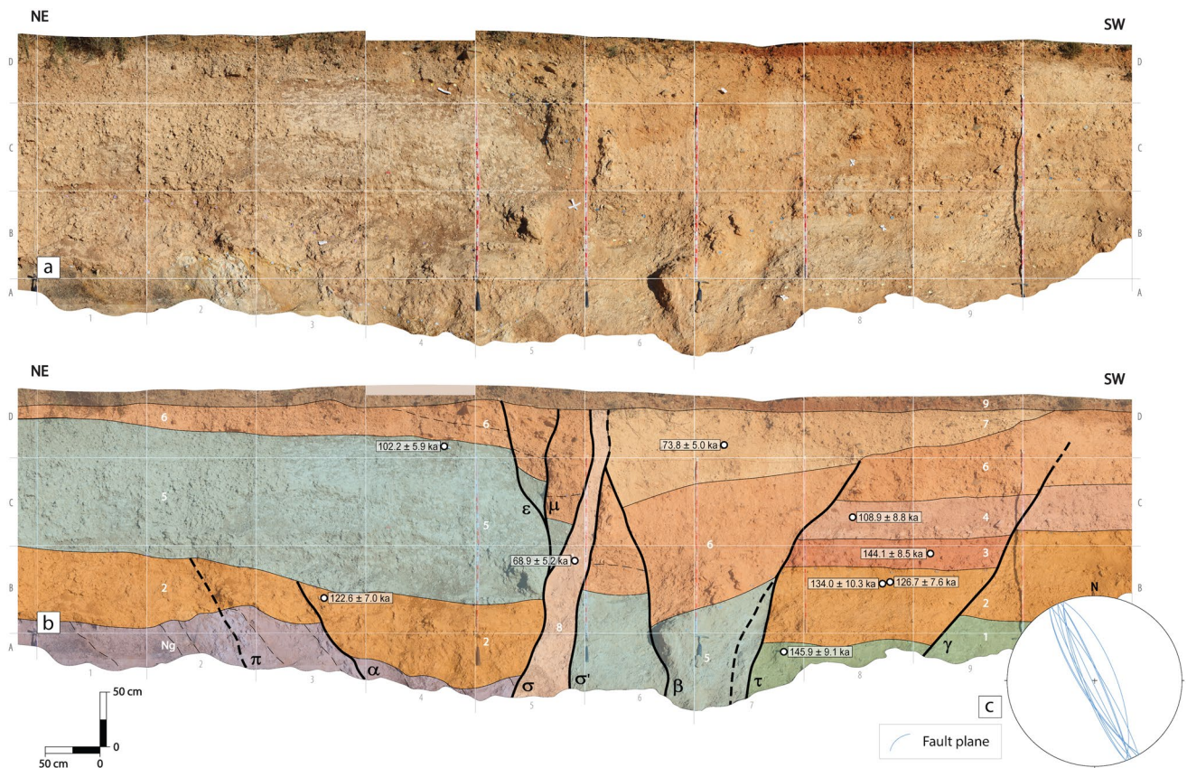
Fig. 9 a Photomosaic of the ZSR trench that crosses branch A; see location in Figs. 4 and 7a. b Detailed log. 1–9: Quaternary units described in the text. Greek characters: faults referred in the text. The
