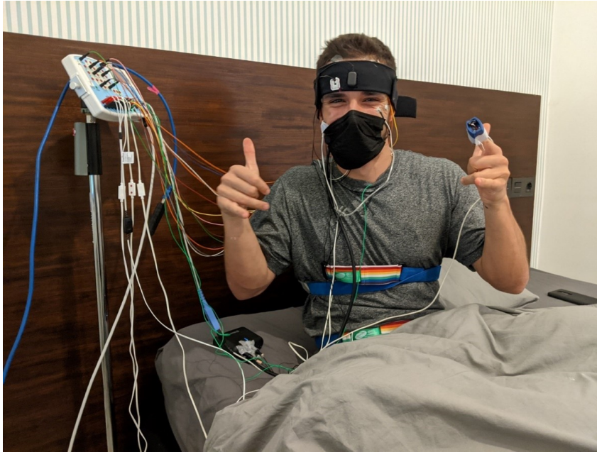
Figure 4.1: Recording setup. Volunteer in one of Bitbrain 's sleep laboratories with a full medical PSG setup and a Bitbrain headband.
