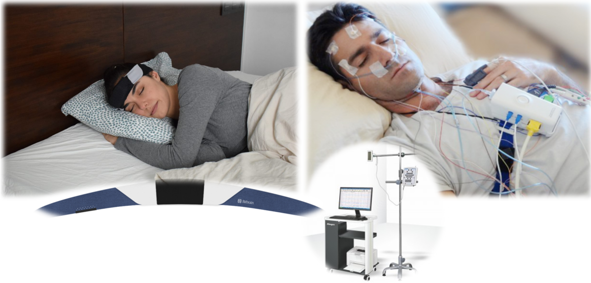
Figure 1.2: Visualization of both types of configuration. Left: PSG, right: wearable 5 EEG channel headband from Bitbrain.
