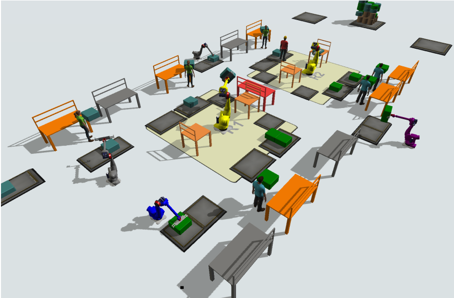
Figure 6.1: Parallel walking-worker assembly line simulation model.
