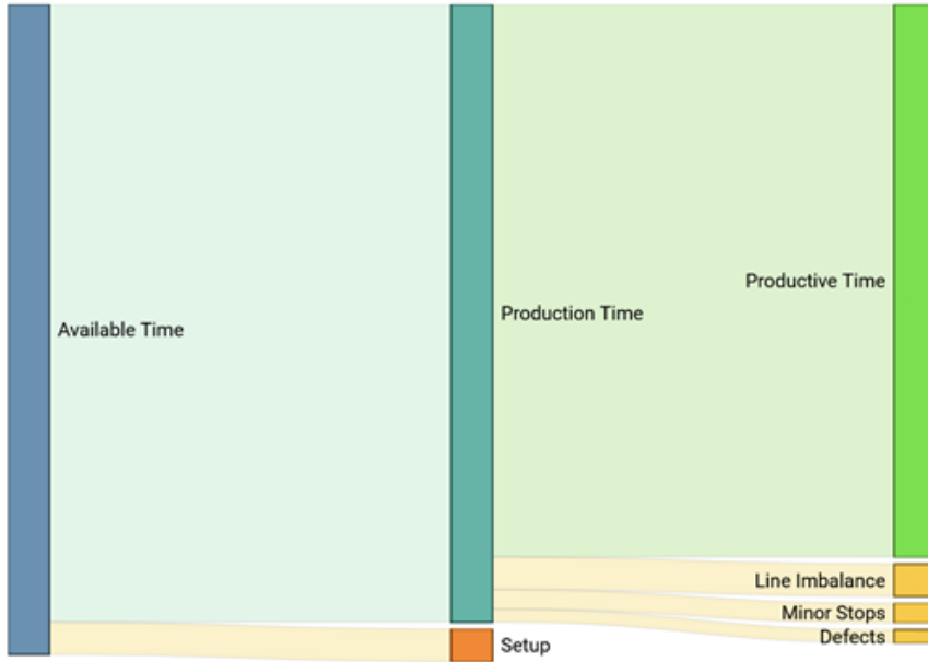
Figure 5.10: Productivity losses in multi-product assembly lines considered in the parametric model.
