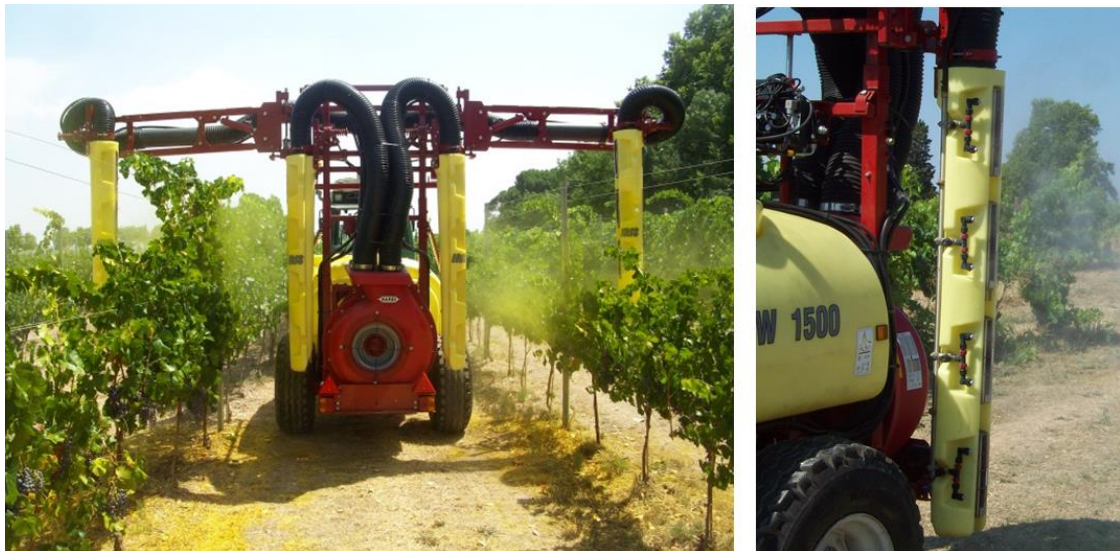
Fig. 1. Multi-row air-assisted sprayer adapted to the vineyard geometry. The centrifugal fan directs the air flow to four vertical ducts (left), each having four air-liquid outlet groups, parallel to the sides of the vineyard line. Each air-liquid outlet group consists of two hydraulic nozzles and four air outlets (right).
