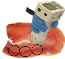
Figure 7. Colorimeter used to measure the colour in the CIE-LAB space.
