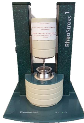
Figure 11. Rheometer used to perform the analysis with the parallel-plates of 60 mm of diameter.
