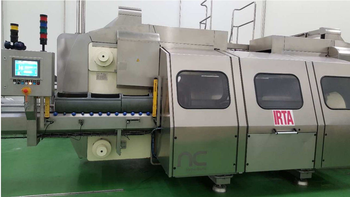
Figure 12. High Pressure Processing machine used for testing.
