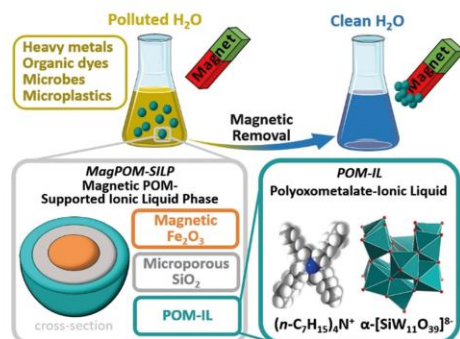
Figure 1. Concept of the removal of multiple pollutants from water using magnetic polyoxometalate supported ionic liquid phases (magPOM-SILPs). Color scheme (bottom right): teal polyhedra [\text{WO}_4] , gray C, red O, blue N, white H.
