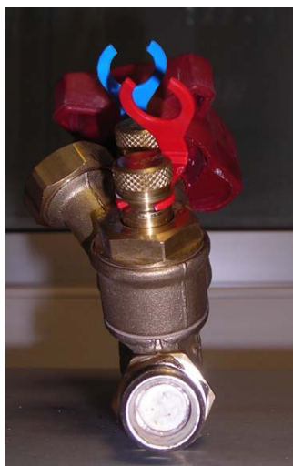
Figure 4.8 Balanced valve of mass flow clogged by the PCM microcapsules from DS 5007 slurry with a mass fraction of 30%.
