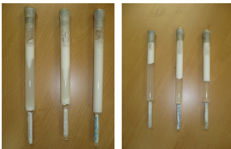
Figure 2.1 Aspect of the slurries prepared from PCM microcapsules. PCM mass fractions 10, 20 and 30%. Left: BASF manufacturer; Right: Microtek Laboratories.
