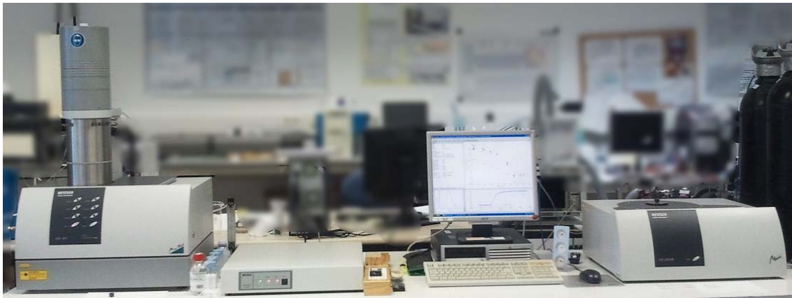
Figure 2.6 Installation of the test bench for the determination of the thermal conductivity of materials in the laboratory for determination of thermophysical properties. Left: DSC; Right: Laser Flash equipment
