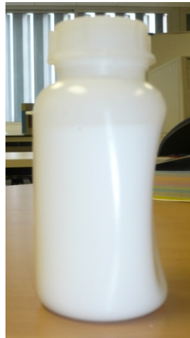
Figure 2.2 Emulsion Fraunhofer UMSICHT with thickener. Deformation of the plastic container.
