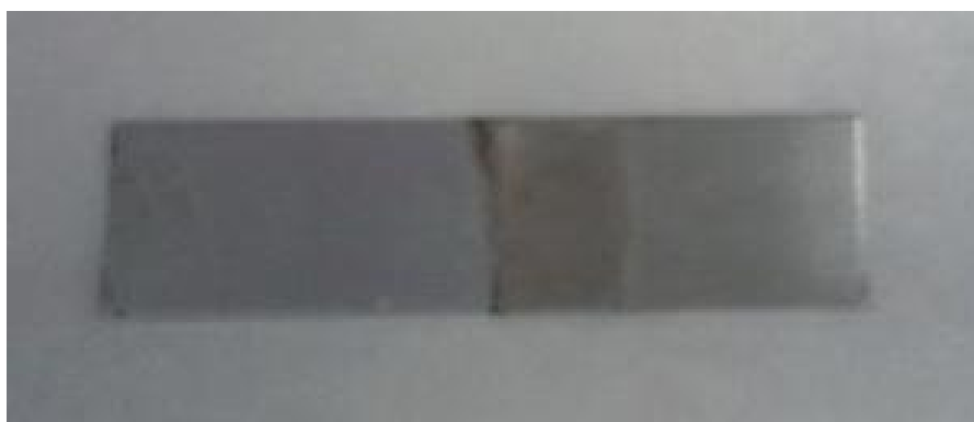
Figure 4.19 Aluminum specimen slightly oxidized.
