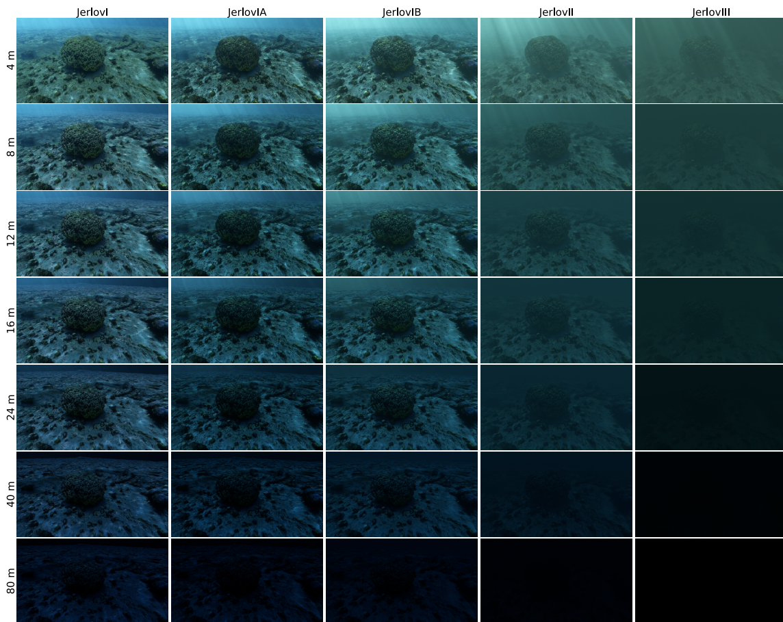
Figure 6.1: Renders of the different Jerlov open waters (I to III), one in each column. The rows show increasing depth.
