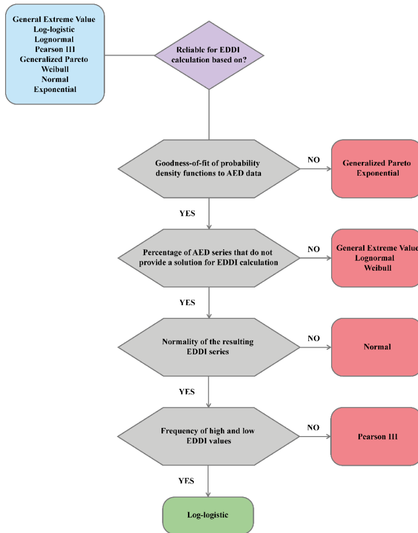
FIGURE 1 Flowchart followed to select the optimal probability distribution to calculate the EDDI [Colour figure can be viewed at wileyonlinelibrary.com]
