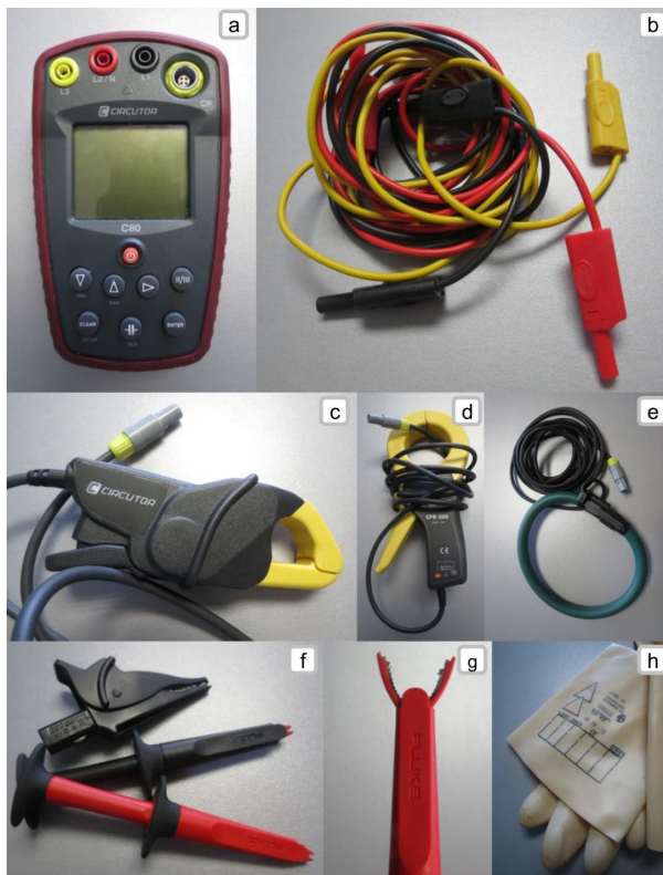
Fig. 1 Measurement equipment: a: Energy monitoring device, b: Voltage wires, c, d, e: Clamps, f, g: Crocodile clamps (for voltage wires), h: Security gloves
