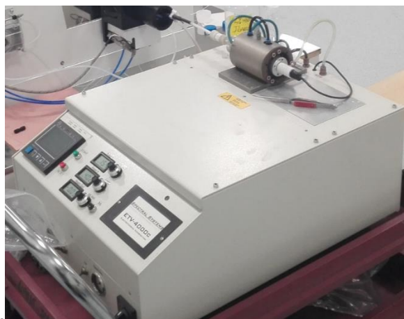
Figure 8. Electrothermal vaporization device (ETV) from Spectral Systems, Fürstenfeldbruck, Germany.
