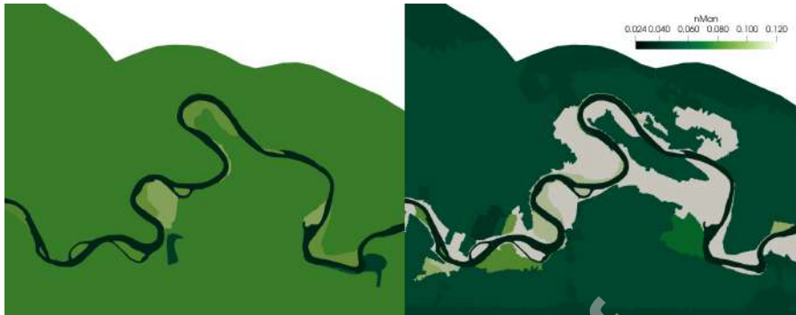
Figure 13: Initial rough (left) and final detail (right) roughness map.
