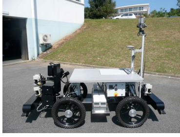
Fig. 3: Robucar-TT platform equipped with IMU, odometry, three range-finder sensors and GPS receiver
