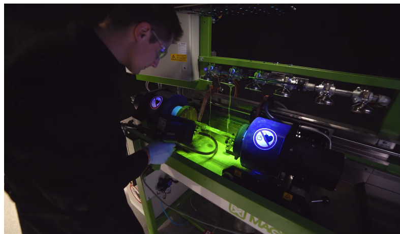
Fig. 1.10: A figure of the MPI performed by the skilled inspector
