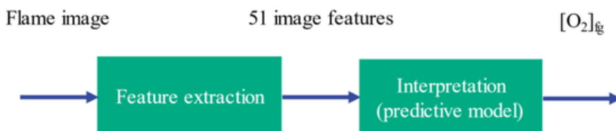
Fig. 3. Method for the processing of flame images.
