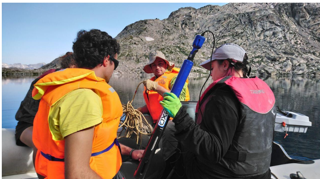
Fig 2.1. Using the YSI EXO1 multiparametric probe in the field
