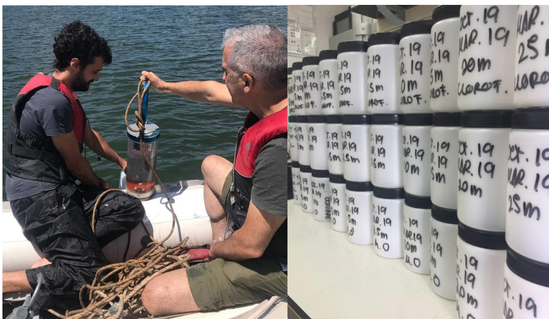
Fig 2.2. Left, collecting water samples with the Niskin bottle in field. Right, sampling bottles with labels.
