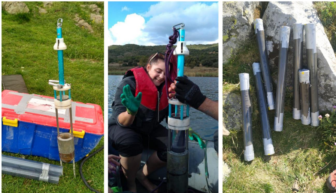
Fig 2.6. Photographs of the Uwitec® gravity corer, the recovery of a core from the boat and a series of recovered cores.
