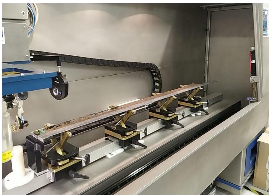
Fig 2.10. Avaatech X-Ray Fluorescence (XRF) from the XRF-Core Scanner Laboratory of the University of Barcelona (UB, Spain)
