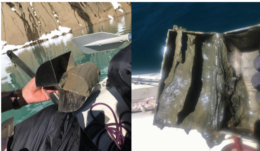
Fig 2.8 Sampling surface sediments with a dredge in Marboré.
