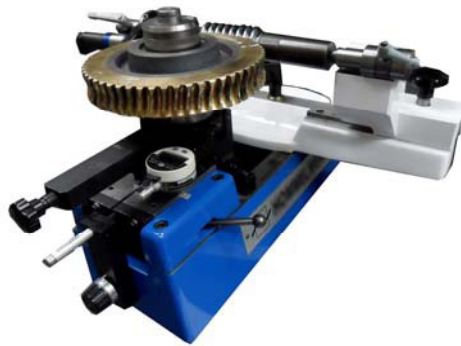
Fig.1. Double flank roll tester for worm – worm gear
