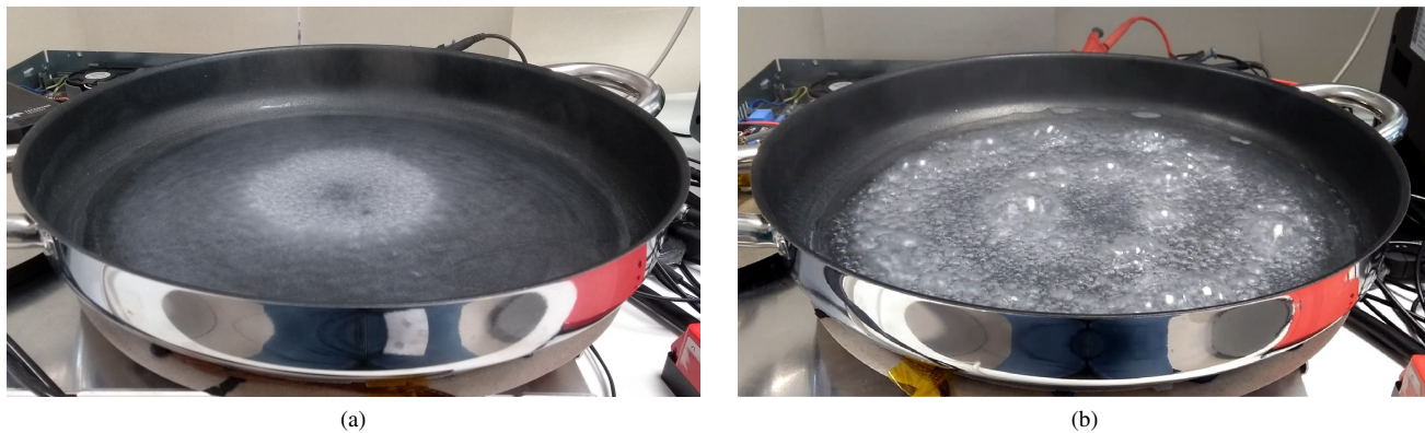
Fig. 18. Water boiling at high power with secondary inductor (a) off and (b) on.
