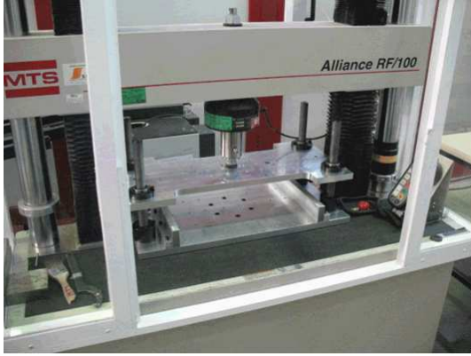
Figure 1: (Color online) Experimental system used for the characterization and the squeeze-flow tests.
