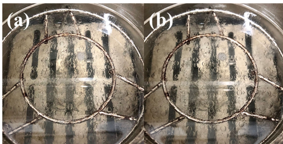
Fig. 3.5 SiO 2 sol dropping spheres in PDMS at 80°C.
