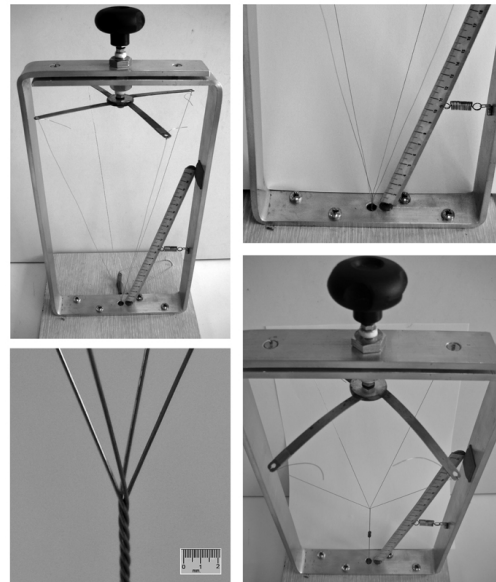
FIG. 1. Sample holder construction nesting the sample inside. The rule at the right side is used for positioning of sample at 4 cm.
