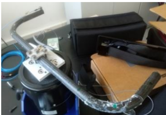
Fig. 4. Vibration test set-up: (left) shaker set-up with carbon prototype, (right) numerical model.
