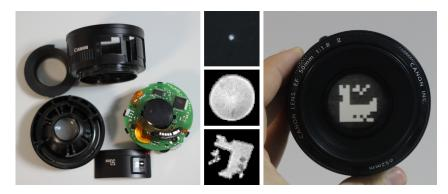
Figure 2.1: *Left:* Disassembled Canon EOS 50mm f/1.8 used in our tests. *Middle:* Point spread function for different apertures and degrees of defocus (*from top to bottom:* circular aperture, focused; circular aperture, defocus depth = 90cm; and one of our coded apertures, defocus depth = 80cm). *Right:* The lens with one of our coded apertures inserted.
