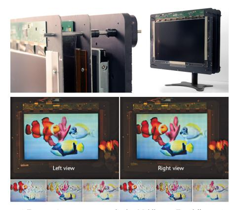
Figure 4.26: Top row: A prototype tensor display. Middle row: Two different views of a light field as seen on the tensor display. Bottom row: Layered patterns for two different frames [478].
