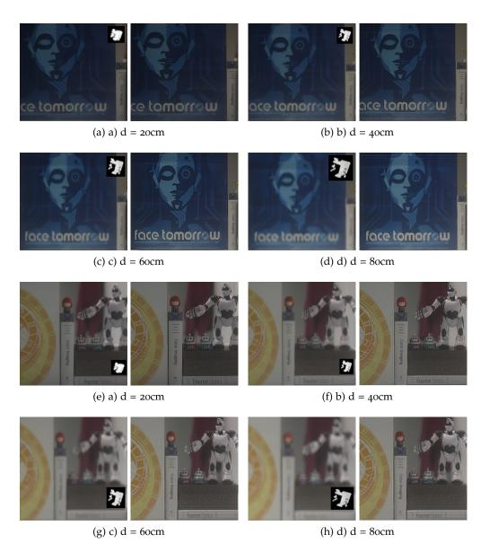
Figure 2.10: Defocused and recovered images at four different defocus depths d obtained with the perceptually-optimized binary coded aperture for two different scenes.
