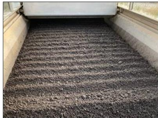
185 Figure 1. (left) Pilot-scale solar drier of SS outside photo (right) Pilot-scale solar drier of SS inside 186 photo
