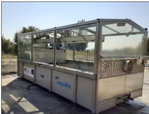
185 Figure 1. (left) Pilot-scale solar drier of SS outside photo (right) Pilot-scale solar drier of SS inside 186 photo
