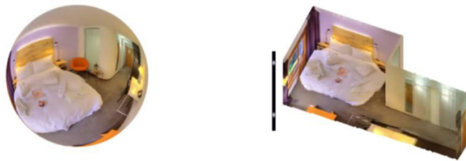
Ilustración 2 Corners for Layout. The model end-to-end predicts the layout corners from the spherical image. Connecting the corners and assuming ceiling-floor parallelism, we can directly obtain the 3D layout in a very short time.
