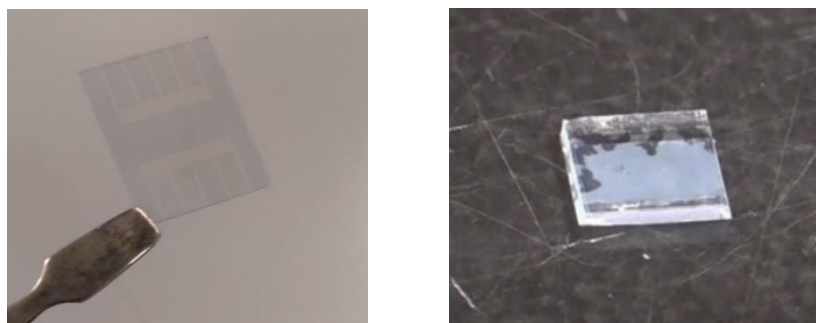
Figure 9.: Left) Laser patterned FTO substrate. Right) Chemically patterned FTO substrate.
