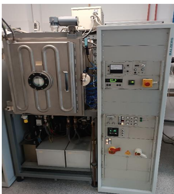
Figure A5.: Left) Thermal evaporator used for gold electrode deposition. Right) Thermal evaporator metallic boat which generates evaporated gold.
