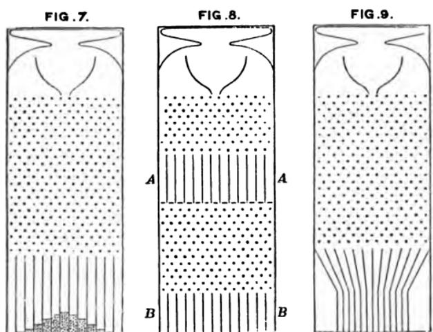
on which Deviation depends. It is a frame glazed in front, leaving a depth of about a quarter of an inch behind the glass. Strips are placed in the upper part to act as a funnel. Below the outlet of the funnel stand a
