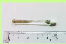
Figure 3. Longitudinal-section view of the Ca 3 Al 2 (SiO 4 ) 3 glass sample grown by the LFZ Technique.
