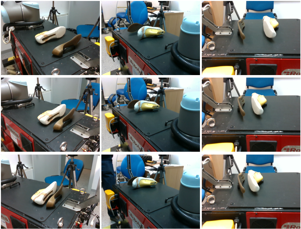
Figure 3.12: Views of three cameras (left to right) in a full visibility coverage experimental setup, where we represent three steps (top to bottom) of a sole-last assembly task.
