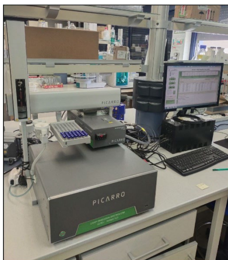
Fig 3.5. PICARRO L2130-i for stable isotopes in water sample analysis.
