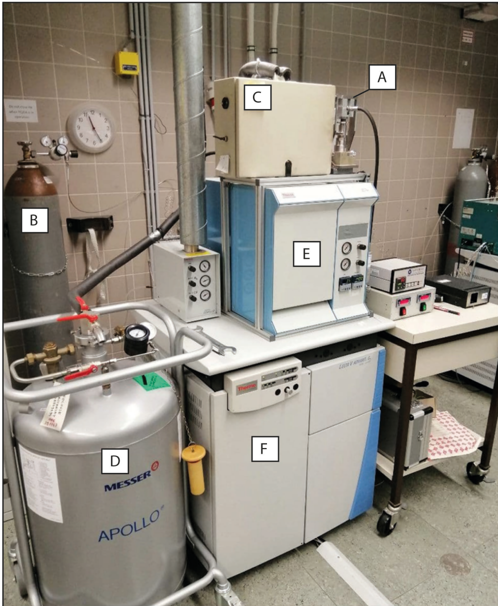
Fig 3.10. Illustration of different steps and devices necessary for the analysis of fluid inclusions used in this study. (A) The sample inside the crusher was pulverized at a high temperature, releasing water from the fluid inclusion that was transported through the He carrier (He comes from a (B) cylinder connected to the crusher) to the cryofocusing cell inside the (C) gas interface housing, which was at very low temperatures owing to the contribution of (D) LN 2 . The sample was rapidly heated to very high temperatures and transported to (E) TC/EA, where molecular hydrogen and carbon monoxide were separated. Finally, molecular hydrogen was analyzed using a (F) Delta V Advantage isotope ratio mass spectrometer.
