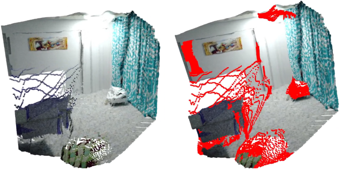
Figure 2.9: Left: Single-view reconstruction. Right: Same reconstruction, with the 10% most uncertain points plotted in red. These points corresponds to spurious or high error points that will degrade the performance of ICP.
