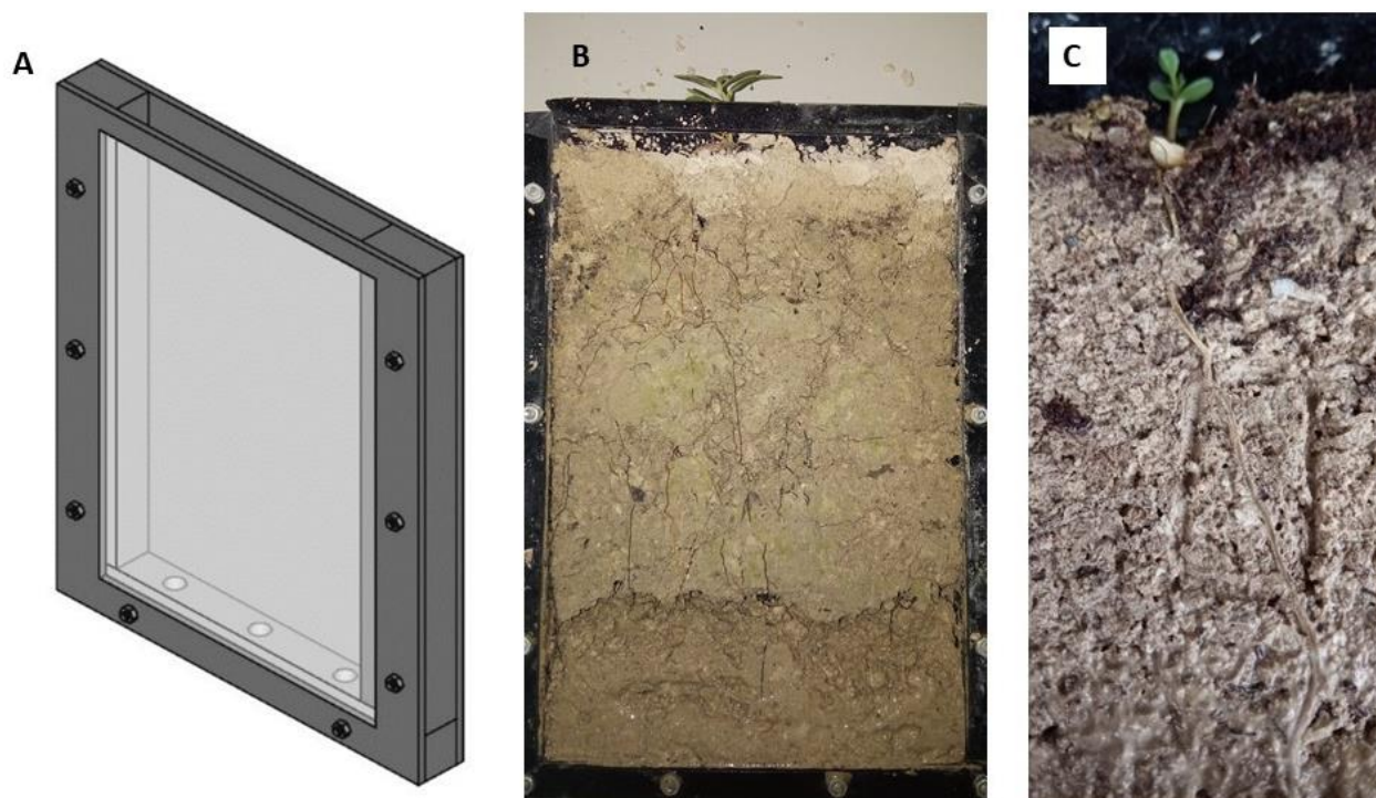
Figure G.M.6. A. Diagram of the rhizoboxes used in the experiment. Designed by Jesus Revilla (Instrument Lab, IPE-CSIC) for this Thesis and inspired by Marschner and Römheld (1983). B. Picture of a H. squamatum seedling after several weeks growing on a rhizobox on gypsum soil. C. O. tridentata seedling growing on a rhizobox on gypsum soil.
