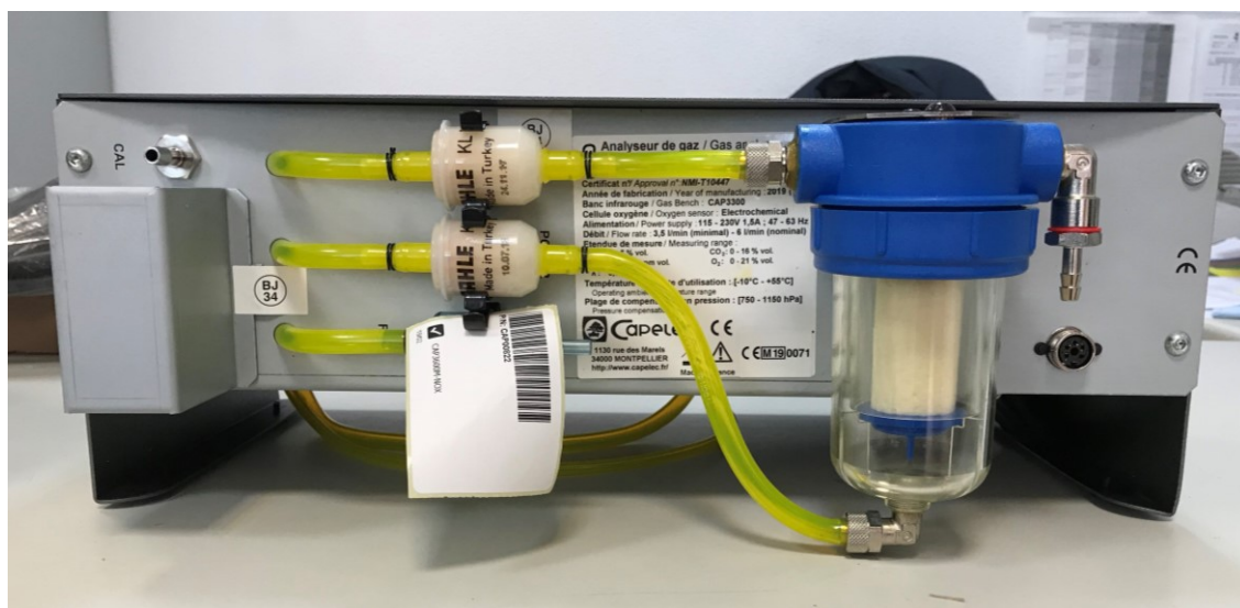
Figure 11-8. CAPELEC Gas Analyzer model CAP3010+S
