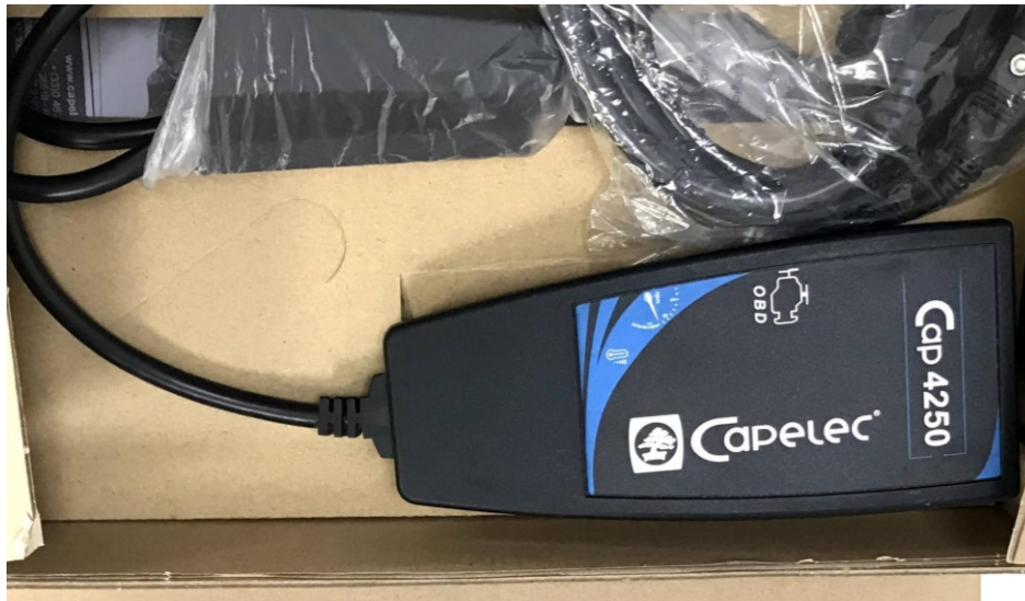
Figure 11-g. CAPELEC interface EOBD CAP 4250+S
