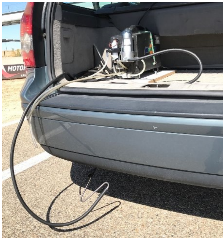
Figure 7-10. Measurement equipment installed into the trunk of vehicle No. 1.
