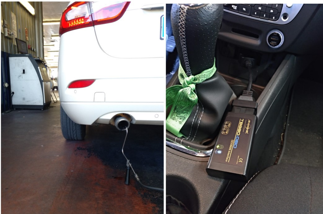
Figure 4-3. Gas analyzer probe into the exhaust pipe, and OBD reader connected.
